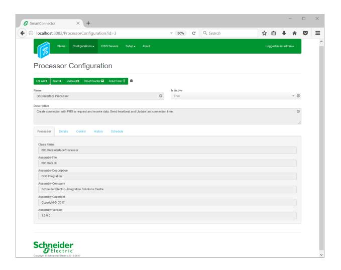
In the configuration window select the Details Tab, you will then be presented with the screen to enter the configuration information. Much of the configuration has default options however they should be checked and validated for the installation. Edit the applicable fields as follows.
