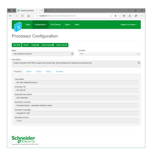
In the configuration window select the Details Tab, you will then be presented with the screen to enter the configuration information. Much of the configuration has default options however they should be checked and validated for the installation. Edit the applicable fields as follows.
