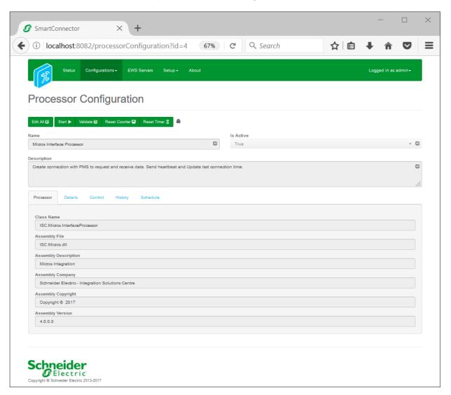
In the configuration window select the Details Tab, you will then be presented with the screen to enter the configuration information. Much of the configuration has default options however they should be checked and validated for the installation. Edit the applicable fields as follows.
